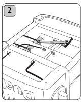
Loosen locking nuts on Unscr retaining plate using a 6.5mm wires. spanner and slide back.
